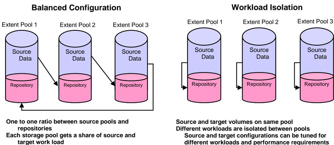
Figure 1 – FlashCopy SE Repository Recommended Configuration Alternatives
