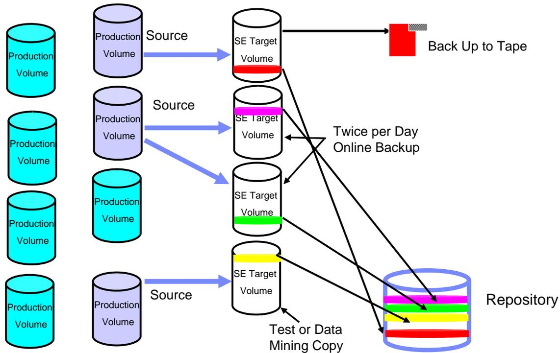
Figure 3 - FlashCopy SE Use Case Example, Backup/Test/Data Mining
