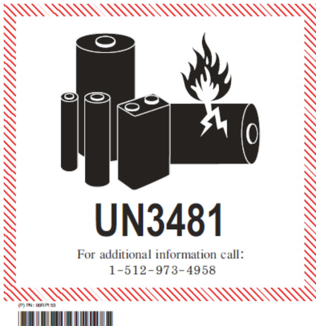
Figure 2 - Example of a Lithium Ion Battery Mark (UN3481) IBM PN 00RP153
