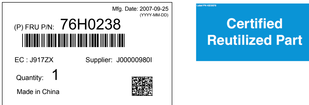
Figure 9 : FRU package label for an ETN non-serialized single item FRU and its companion 'Certified Reutilized Part' label (PN 45D3078)
