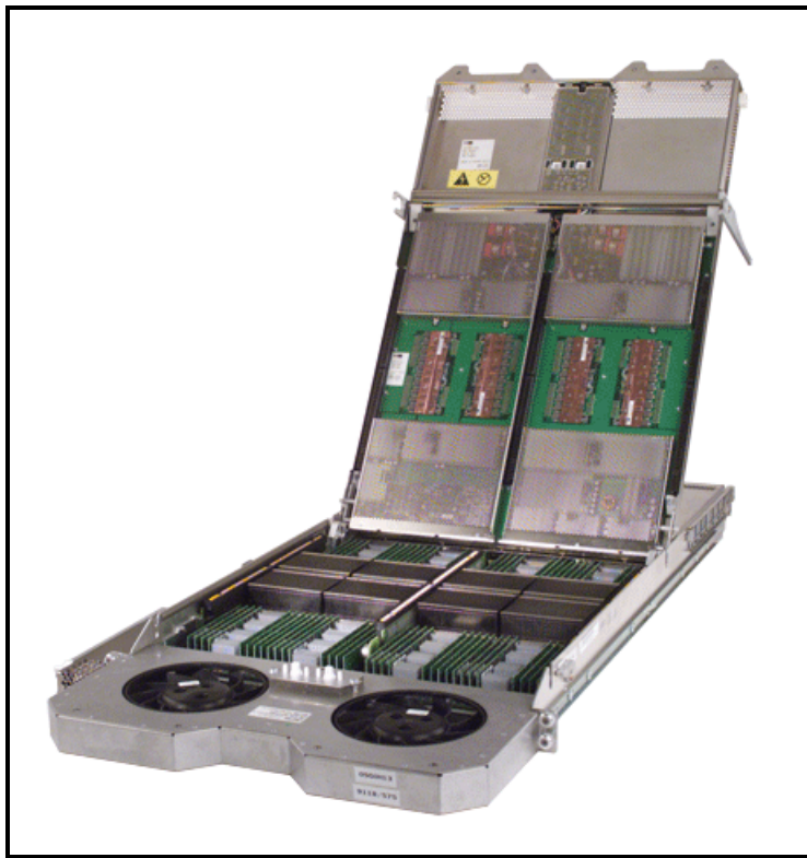
Figure 1: p5-575 Case Opened to Show CEC and Fans
