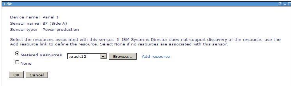
Figure 7: Configure Metering Device (Associate resource to Sensor)
