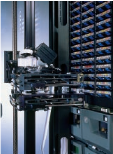
The Magstar 3494's cartridge accessor with the dual gripper feature provides increased performance and availability.
