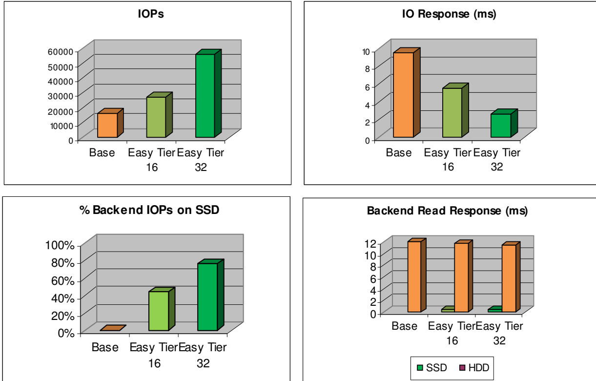
Figure 10: Backend Storage Measurements at Queue Depth 20.
