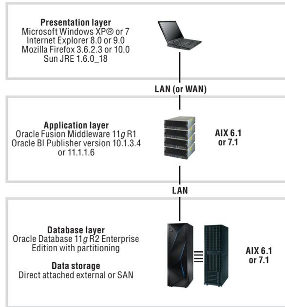
Figure 2. Hardware and software architecture for RMS 13.2.5
