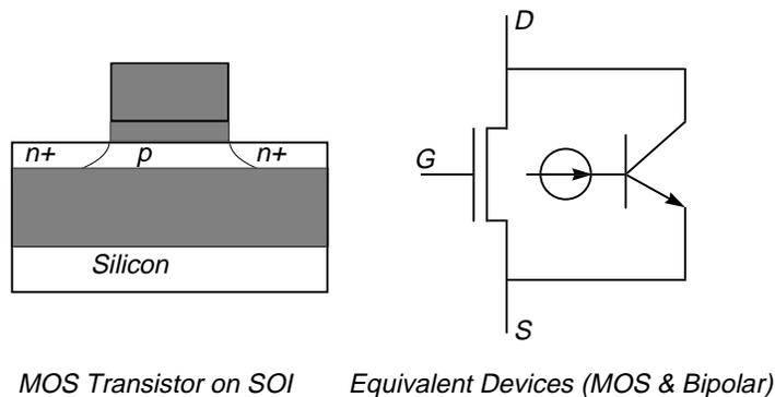
the operation of the chip's circuit and its modeling. Significant effort has been devoted in the last three decades in characterizing, modeling, eliminating or at least reducing, and controlling the unwanted effects caused by the bipolar device.
