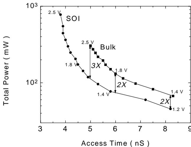
\*Note: Performance characteristics displayed above are actual figures derived in lab tests using SOI-based chips
