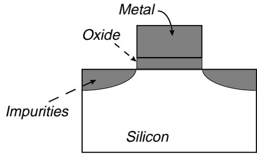
On the piece of silicon that is on either side of the metal, known as a “gate” area, chemical “impurities” are added to make the silicon conduct electricity. If current is transmitted to the metal, the silicon will conduct electricity. The “impure” silicon will be “attached” to the two conducting areas on either side of the metal and electricity will flow. Silicon, then, can act both as a conductor and a non-conductor, which is why it is called a “semi-conductor”.
