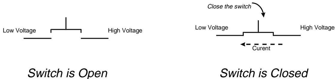
The switch that is used to turn a light on and off is very big, very slow, and carries a lot of current. The transistor or "electronic switch" is usually very small, very fast, and carries less current. There are two basic type of transistors or electronic "switches" -- bipolar and MOS or metal-oxide-semiconductor.
